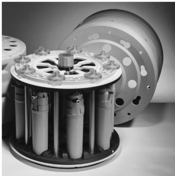
Figure 2. View of the eight-position rotor system. Visible are the protecting air cooling jackets made of PEEK containing the quartz or PTFE-TFM vessels and the pressure release valves. The protection hood is shown in the back. This rotor system is placed in the cavity of the reactor.
